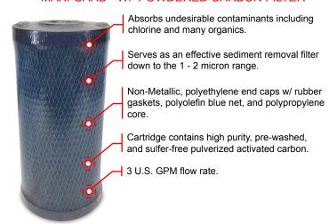
Designed to fit SERFILCO GPO10-1 chamber. See Bulletin C-101
