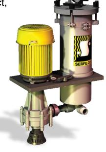
SERFILCO® products have gained global approval for recirculation purification of most electroplating and chemical process solutions. They have proven to be a reliable workhorse for over half a century.
